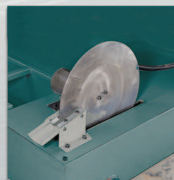
OP. 油水分離機 Oil skimmer: Eco-friendly coolant disposal system
