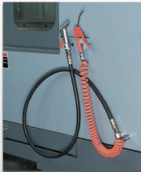
風槍水槍 Powerful air and wash down gun are conveniently built-in
