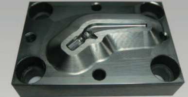
Medical Instruments Mold Machining * Workpiece name:Artificial bone mold * Workpiece material:SKD61(HardnessHRC50) * Workpiece :SKD61(HardnessHRC50)
