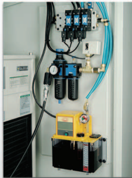
三點組合 Equipped with high reliability lubrication pump and solenoid valves.
