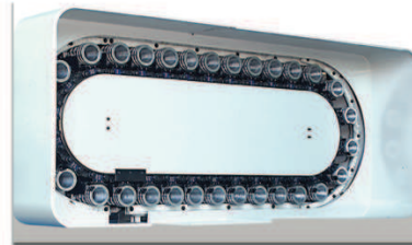
OP:高容量刀庫(40刀) Chain type ATC
